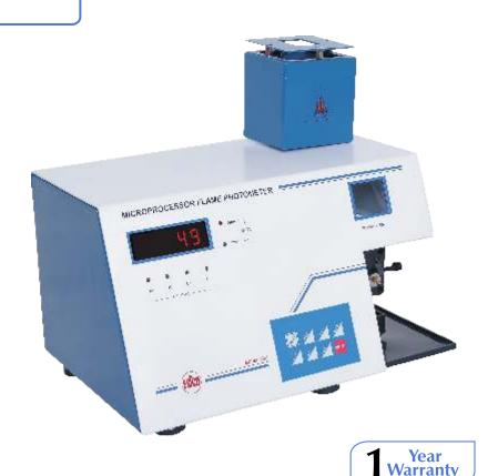
MICROPROCESSOR FLAME PHOTOMETER, MODEL 1381 is an ideal instrument for the determination of Sodium, Potassium, Calcium and Lithium. It uses the latest Microcontroller technology and advanced engineering techniques so as to give enhanced accuracy and reproducibility. The System has 3 point calibration facility using curve fitting software. It has soft
